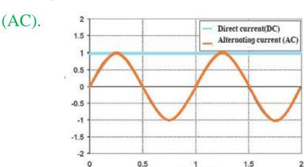
Electric current changes sinusoidally with time Electric current and potential difference are shown by the symbol ~
