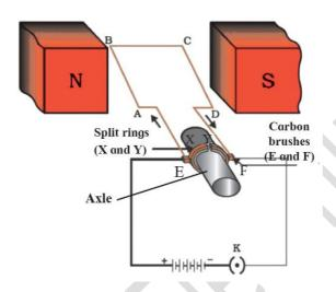
Working: (1) When the circuit is completed with a plug key or switch, the current flows in the direction E - A - B C - D - F. As the magnetic field is directed from the north pole to the south pole, the force on AB is downward and that on CD is upward by Fleming's left had rule. Hence AB moves downward and CD upward. These forces are equal in magnitude and opposite in direction. Therefore, as observed from the side AD the loop ABCD and the axle start rotating in anticlockwise direction.
