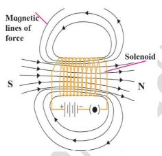
The magnetic field lines (magnetic lines of force) due to a current-carrying solenoid solenoid are similar to those of a bar magnet. One face of the coil acts as the south pole and the other face as the north pole.
