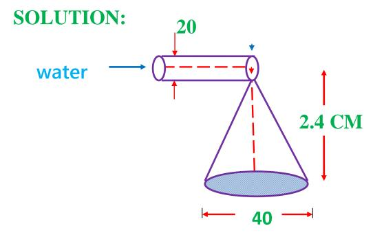
Diameter of Cylindrical shape pipe = (D) = 20 mm Radius of pipe = 10 mm = 1 cm Rate of flow of water through the pipe = 10m/minute h = 1000 cm / minute For conical pot,
