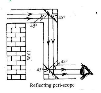
Uses of a Reflecting Periscope -
