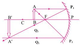
Object placed between focus and centre of curvature
