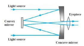
mirror and then through the eyepiece situated at the back of the mirror. The eyepiece gives us a magnified image of the source
