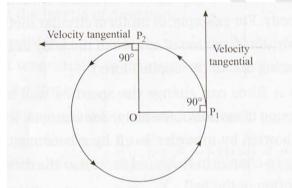
Fig 1.7 : (for reference) : Velocity of a particle in uniform circular motion
