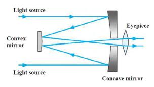
concave mirror and then through the eyepiece situated at the back of the mirror. The eyepiece gives us a magnified image of the source
