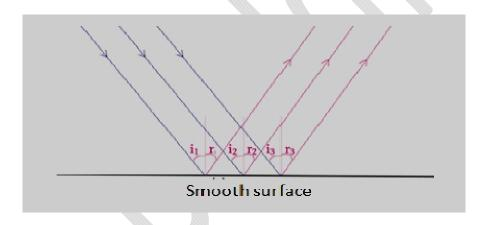
The reflection of light from a plane and smooth surface is called regular reflection of light. For regular reflection, the angles of incidence as well as of reflection are the same for all parallel rays falling on the surface. Thus, the reflected rays are also parallel to one another.
