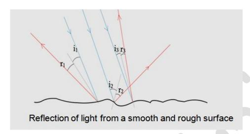
Reflection of light from a rough surface is called irregular reflection of light. In irregular reflection, the angles of incidence for parallel rays of incidence are not equal and therefore their angles of reflection are also not equal.
