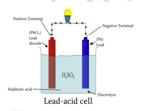
The lead-acid cell (pb) contains a lead electrode and a lead oxide electrode (pbo<sub>2</sub>) and both are dipped in dilute sulphuric acid. pbO<sub>2</sub> carries a positive charge, while the Pb electrode carries a negative charge. The potential difference between these two is nearly 2V. Because of the chemical reaction between the substances in the cell, electrical charge is produced on both the electrodes.
