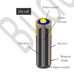
In dry cell, zinc metal acts as negative terminal while carbon electrode acts as positive terminal.
