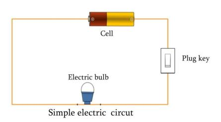
When a cell holder, an electric bulb and a plug key are connected by connecting wires, as shown in figure and dry cell is fitted in the holder, then the bulb lights up by closing the plug key. This means that a current flows through the circuit and bulb lighten up. On the removal of the cell, the electric current flowing through the circuit stops as indicated by the bulb which ceases to glow. This type of connection of electrical components is called as electric circuit.
